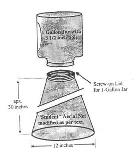
Figure 2. Net to replace lower collecting jar. The tip of the net is cut off, and sewn or glued to the screw cap for the gallon jar. The bottom of the net has a net ring inside to keep it open, and cotton muslin fabric sewn across the opening.
