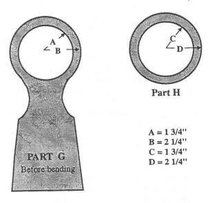
Figure 1. Patterns for the metal parts that connect to the collecting head in the new design. See Townes (1972, Figure 2) for the remainder of the parts and assembly directions.
