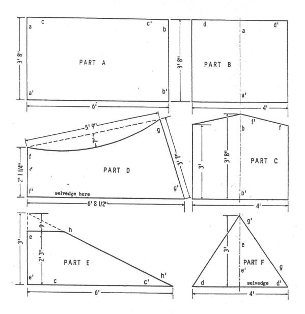
Figure 3. Patterns for the fabric parts of a Malaise trap. Reprinted from "Figure 1" in Townes (1972).
