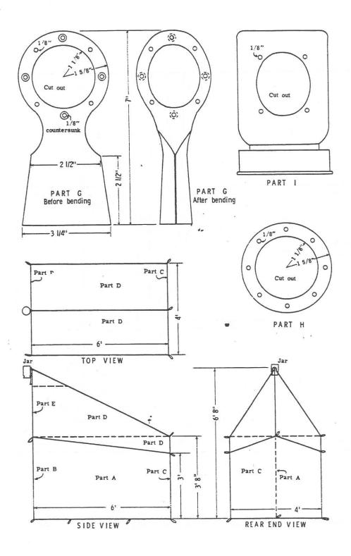
Figure 4. Patterns for the metal parts and modified plastic jar for a Malaise trap. Three views of the complete trap. Reprinted from "Figure 2" in Townes (1972).
