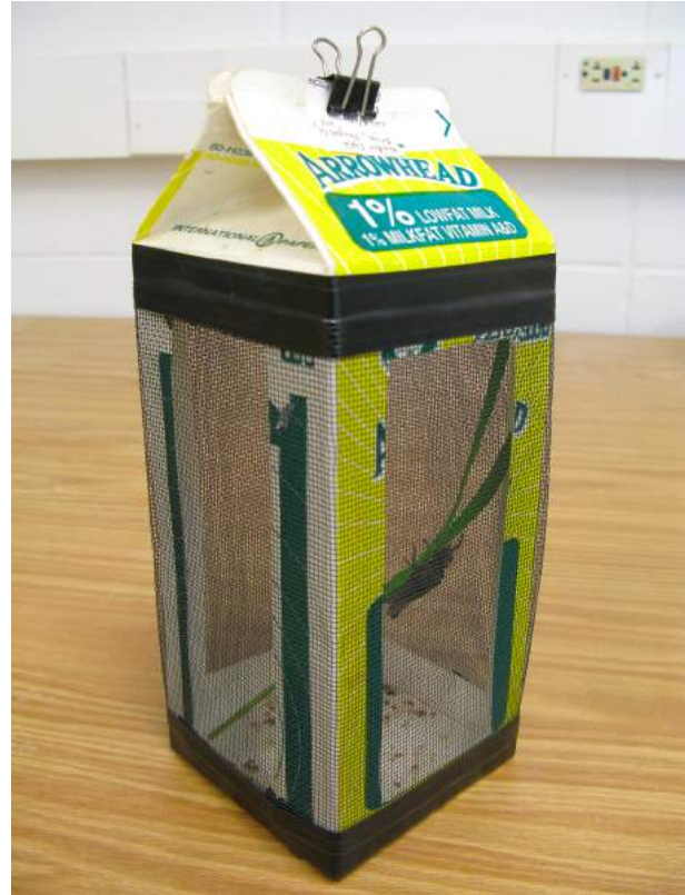
Figure 4. Rearing cage constructed a ½ gallon beverage container and window screening.
